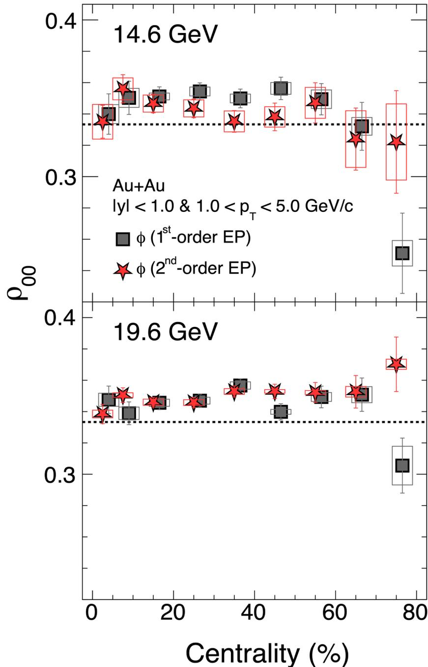
Centrality dependent  $\rho_{00}$  with respect to the first and second order event planes for Au+Au collisions at  $\sqrt{s_{NN}} = 14.6$  (top) and 19.6 (bottom) GeV. The first order event plane results are slightly shifted horizontally. The vertical lines are statistical uncertainties and boxes represent systematic uncertainties. The black dashed line represents  $\rho_{00} = 1/3$ .
