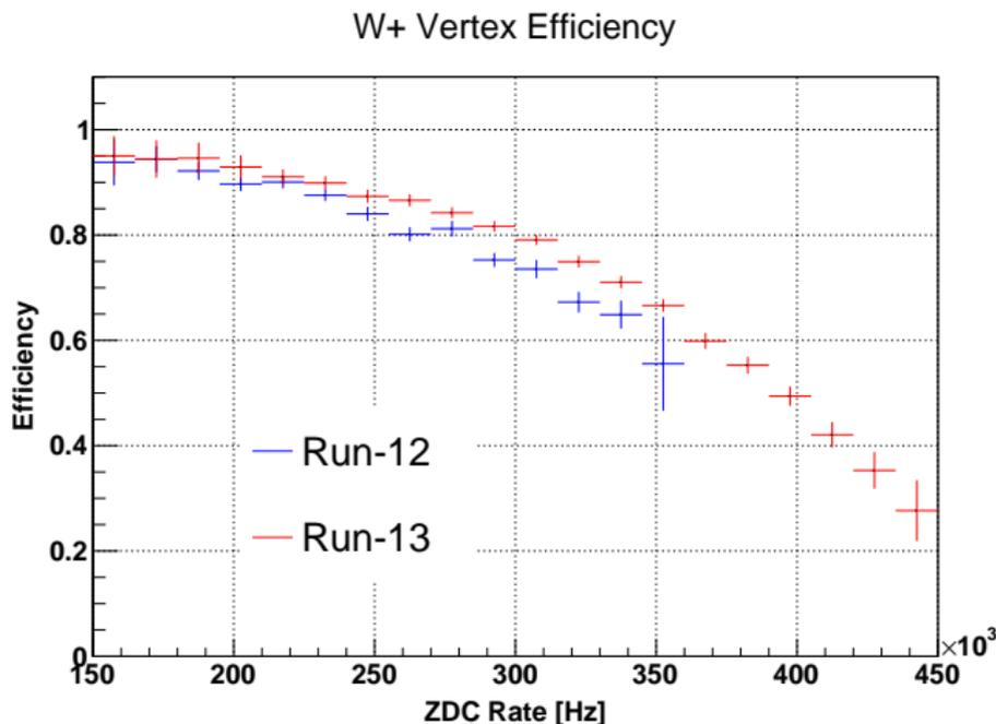
Figure : Run 12 and Run 13  $W^+$  vertex reconstruction efficiency as a function of zdc rate.
