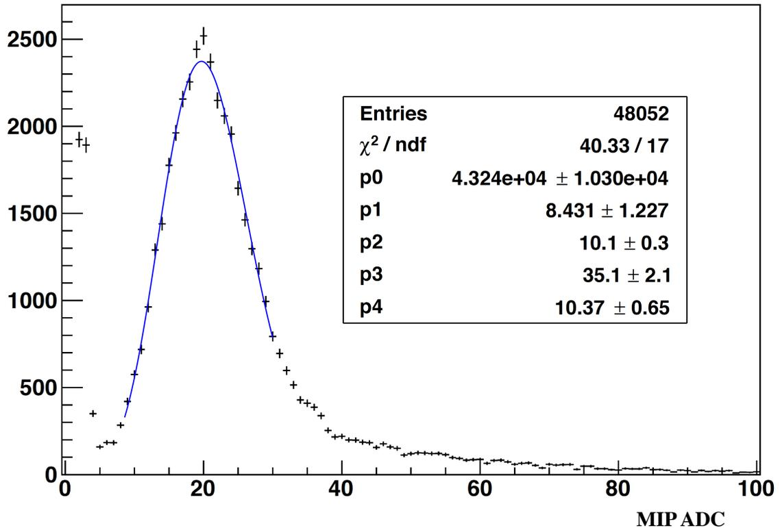
Figure 1: A typical MIP ADC distribution (black points) and gaussian  $\times$  landau fit (in blue) for a single tower.
