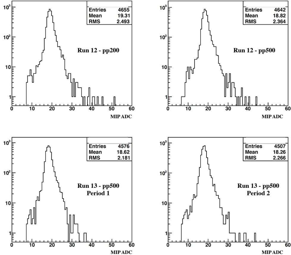
Figure 3: Distributions of the MIP peak values from STAR Run 12 p-p 200 GeV (upper left panel), Run 12 p-p 510 GeV (upper right panel), Run 13 510 GeV period 1 (bottom left), and Run 13 p-p 510 GeV period 2 (bottom right) running periods.
