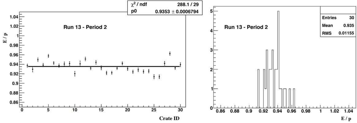
Figure 23: Average  $E/p$  per calorimeter crate for period 2. Left panel  $E/p$  vs. crate ID. Right panel: Spread of  $E/p$  from crate to crate.
