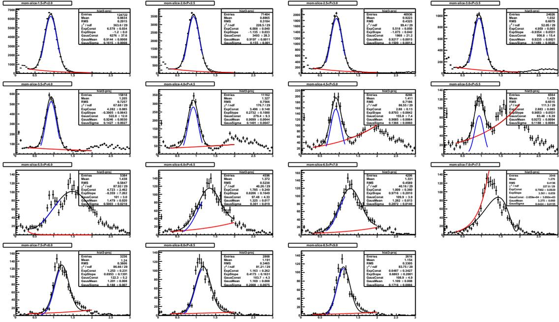
Figure 8:  $E/p$  distributions of momentum slices of width 0.5 GeV of BHT3 trigger events
