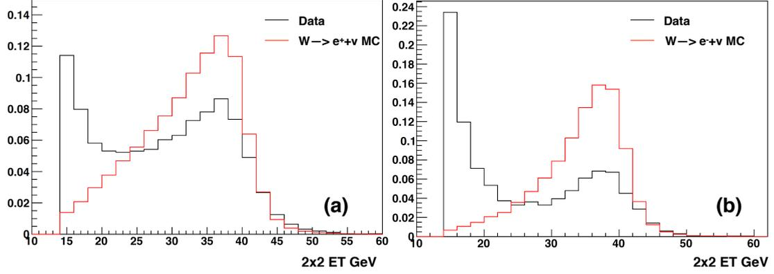
Figure 13:  $E_T^c$  distribution of  $W^+$  (a) and  $W^-$  (b) candidate events (black) from STAR Run 13 data (after run 13 gains applied),  $W \rightarrow e\nu$  MC signal (red).
