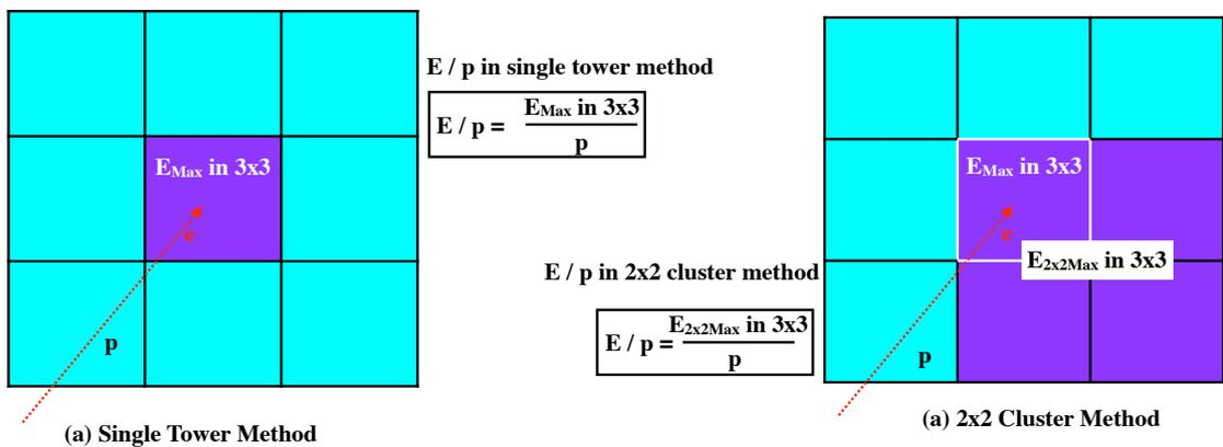
Figure 5: Methods used in the Run 13 BEMC absolute gain calibration.
