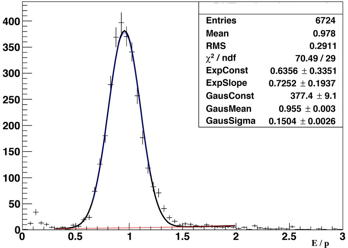
Figure 6: A typical electron  $E/p$  spectrum for one of the eta rings (black points), gaussian fit to the signal region (blue curve), exponential fit to the background region (red curve), and the sum of the two fits (black curve).
