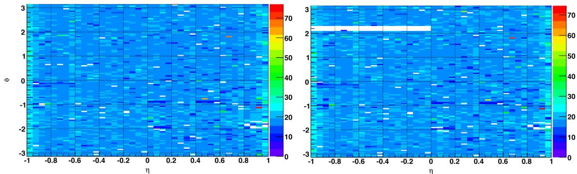
Figure 4: Relative gain constants of the calorimeter towers of Run 13 periods 1(left panel) and 2(right panel).
