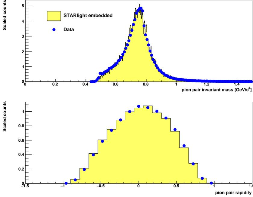
Figure 2: Comparison of uncorrected data (blue points) with embedded simulated  $\rho^0$  and direct  $\pi\pi$  events (yellow histogram). The simulated UPCs were run through a GEANT simulation of the detector, embedded in randomly triggered (zero-bias) events, and subject to the same reconstruction programs as the data.
